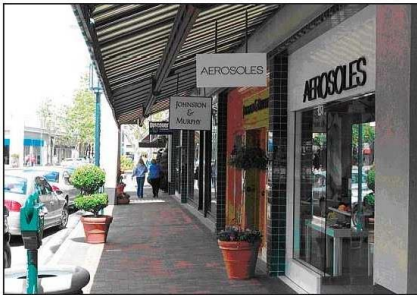
3.2.3.7 h) Signage in town centers should be oriented to the pedestrian. Double-faced hanging signs, wall signs and awnings are all scaled to the pedestrian
