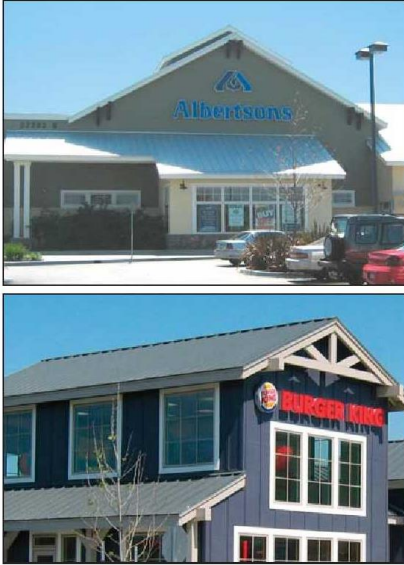
3.3.3.3 a) Exposed rafter ends, overhanging eaves, multiple roof planes and varied fenestration create interesting commercial buildings.
