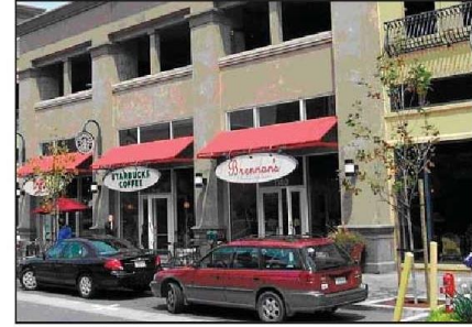
3.2.3.7 e) Awnings, signs and lighting help reduce the bulk of a building and create a pedestrian scale environment..
